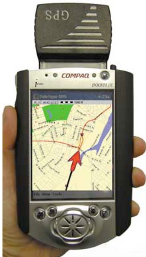
Figure 4: iPaq PDA with GPS extension.
